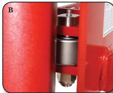
Roller bearings make mast rotation easy and smooth.
